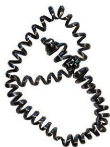
Stringy, uninterrupted chips without Oscillation Cutting.
