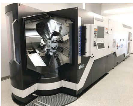
(left and right) The MultiSwiss 8x26 on display at the grand opening event. It is equipped with eight spindles and eight slides for main operations, and housing up to three tools per slide.
