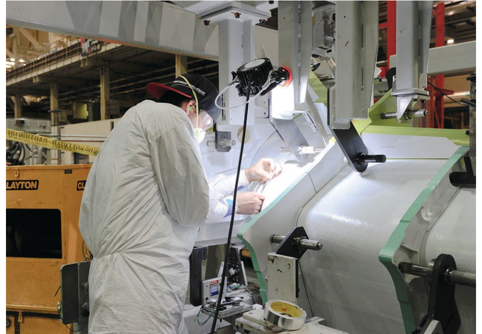
An F-35 technician measures the gaps between the frames and the ducts on the forward left inlet duct for the F-35 center fuselage. A core structure of the F-35 Lightning II aircraft, the center fuselage is produced on Northrop Grumman's integrated assembly line at its Palmdale Aircraft Integration Center of Excellence.
