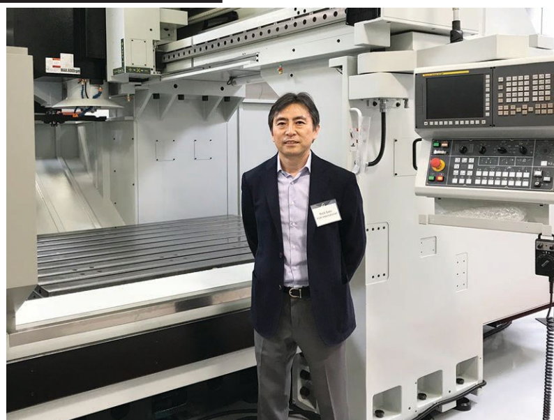
Rich Sato, Account Manager, KGK International, with the Kent KVM-22P Double Column CNC Machining Center. It features a large table size, a 32-tool capacity and a 30 HP multi-speed spindle.
