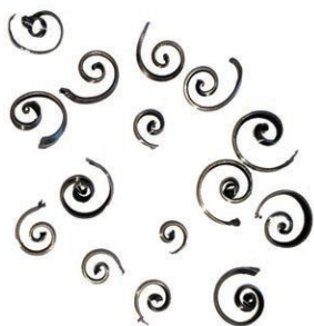
Chip break up with Oscillation Cutting.
