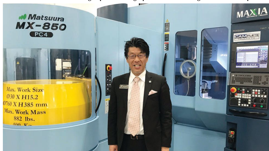
Katsutoshi Matsuura, President, Matsuura Machinery USA with the new MX-850 PC4, an automated version of the large capacity 5-axis vertical machining center featuring 90 tools and a load capacity per pallet of 500kg.
